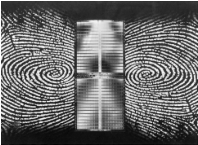
Figure 3. The 16-Megabit Chip: 700 Typewritten Pages on a Fingertip (Siemens Press).
